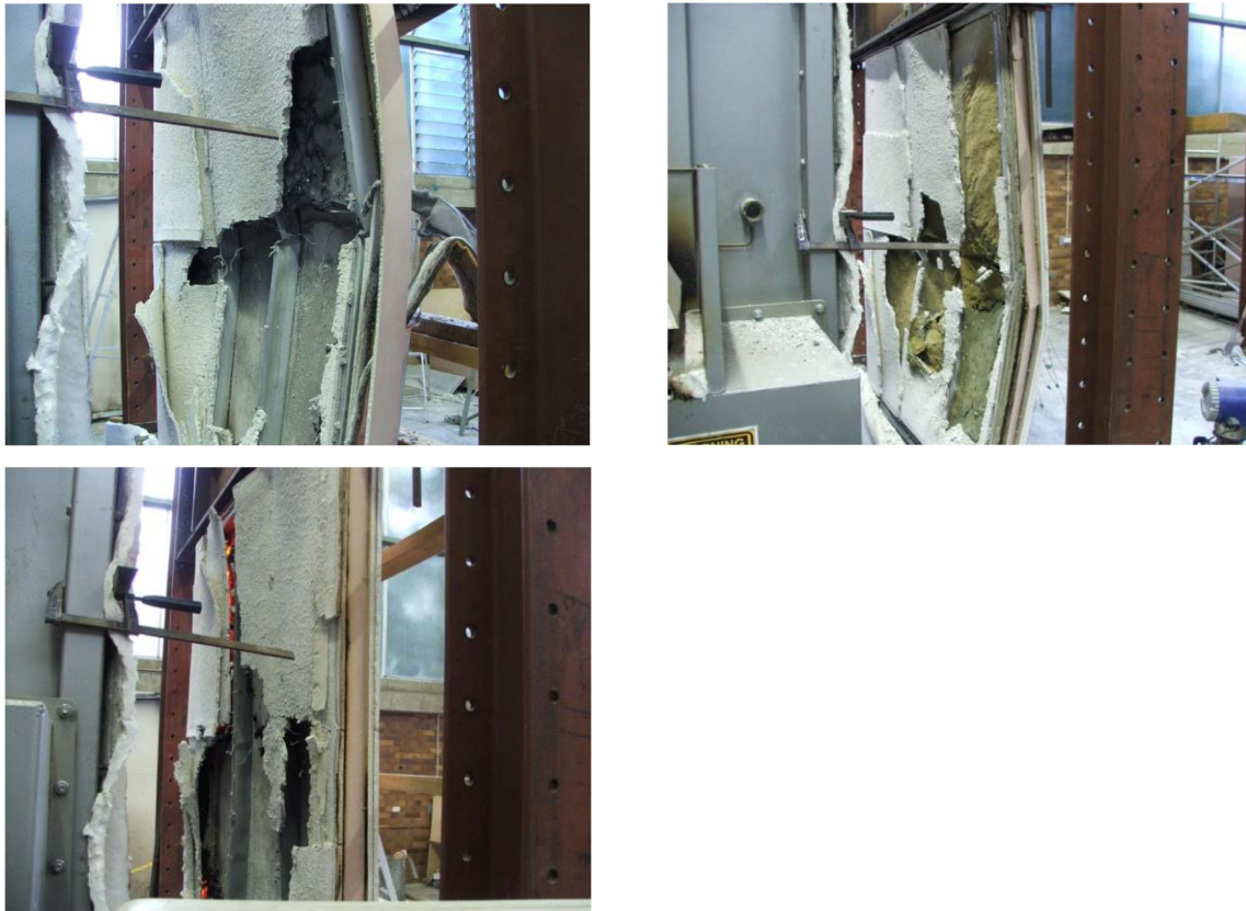
Fig. 28 – Experimental tests for the (a) glass fibre, (b) rock fibre and (c) cellulose fibre cavity insulation made by Kolarkar [41] and studied by Rusthi et al. [40]
