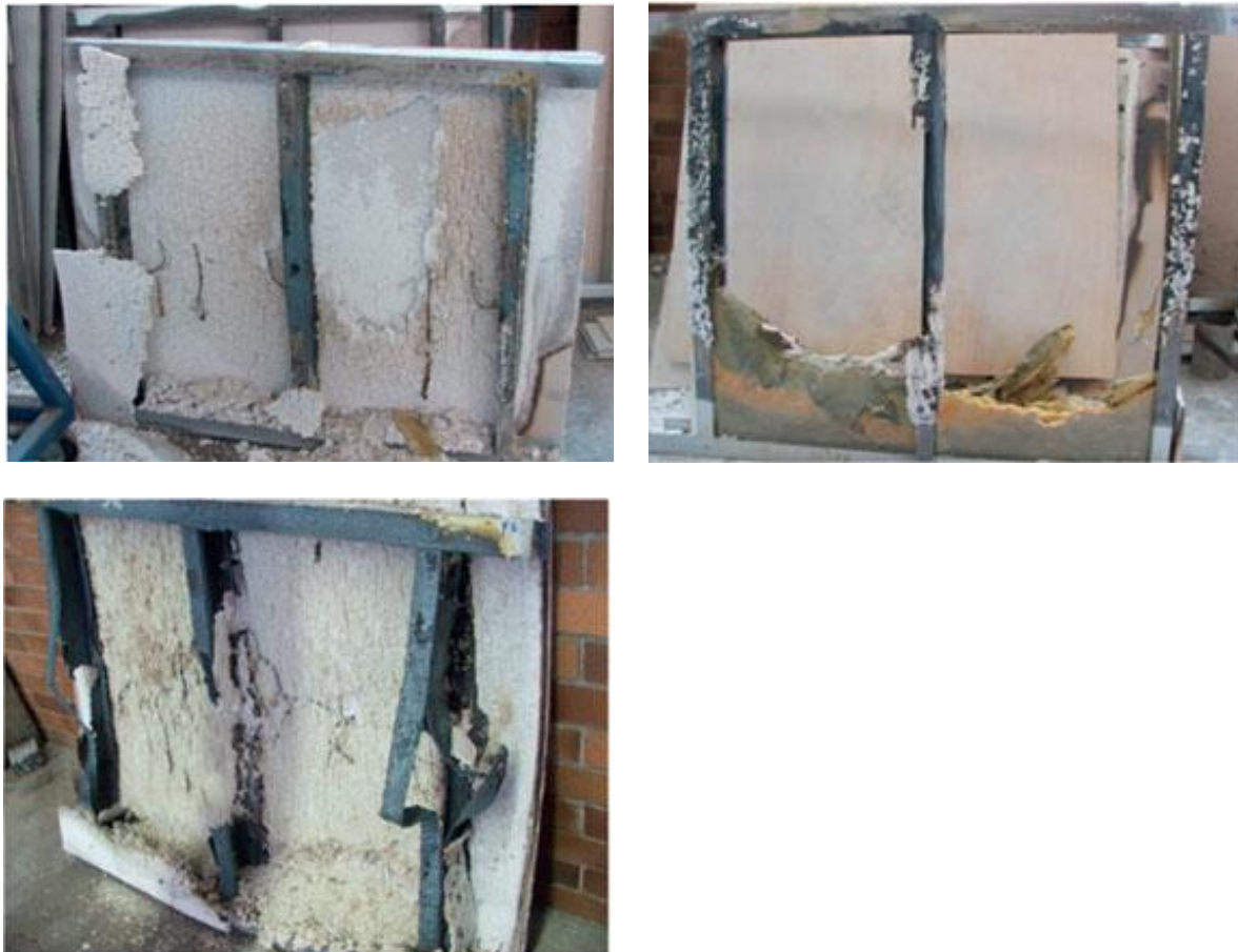
Fig. 27 – Experimental tests for the (a) glass fibre, (b) rock fibre and (c) cellulose fibre cavity insulation made by Kolarkar et al. [39]
