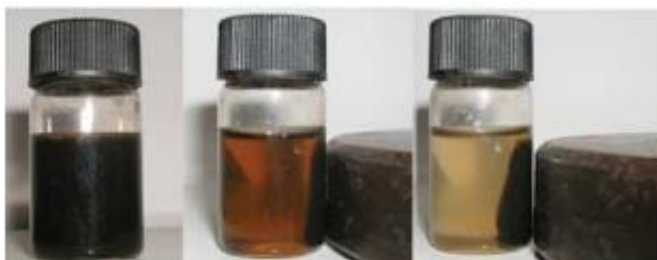
Figure 3. The separation of \text{CoFe}_2\text{O}_4 nanocrystals from the solution by the action of a magnetic force 36
