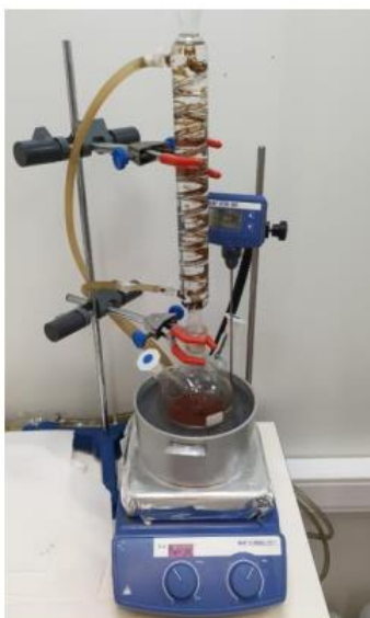
Figure 11. The reaction system used in the CWPO runs
