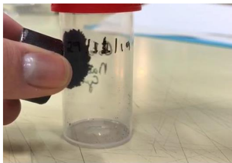
Figure 20. CoFe 2 O 4 @void@C catalysts in the presence of a magnetic field
