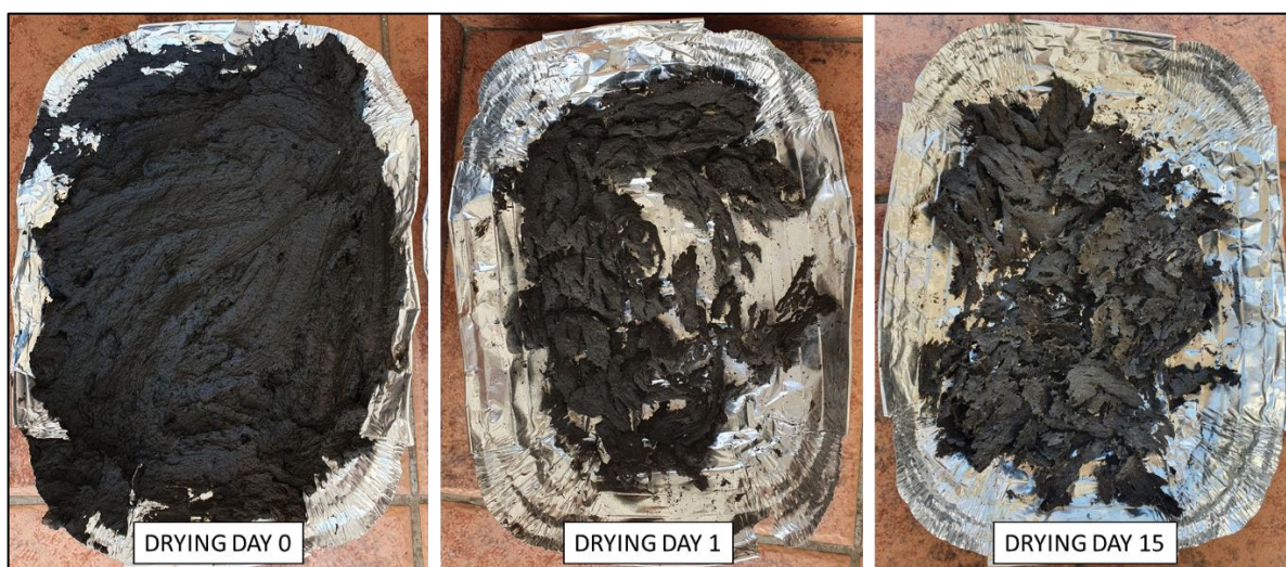
Figure 8: Sun dried sludge samples
