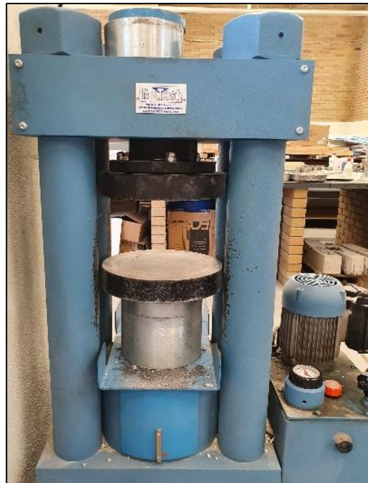
Figure 6: Compressive strength testing equipment
