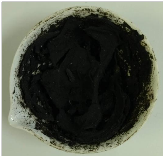
Figure 7: Oven dried sludge sample
