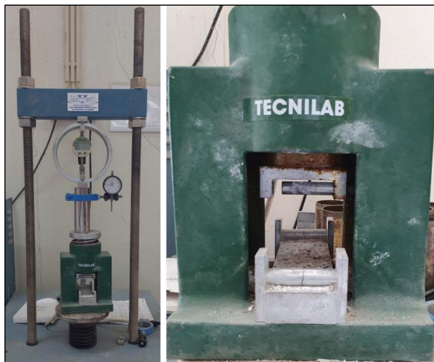
Figure 4: Equipment for testing flexural strength
