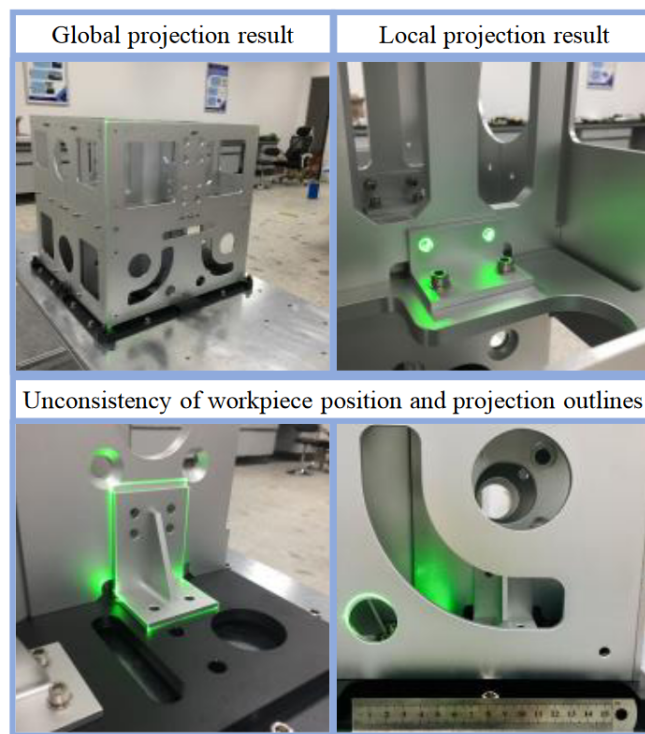
Figure 2.5: Laser projector assisted assembly [45]
