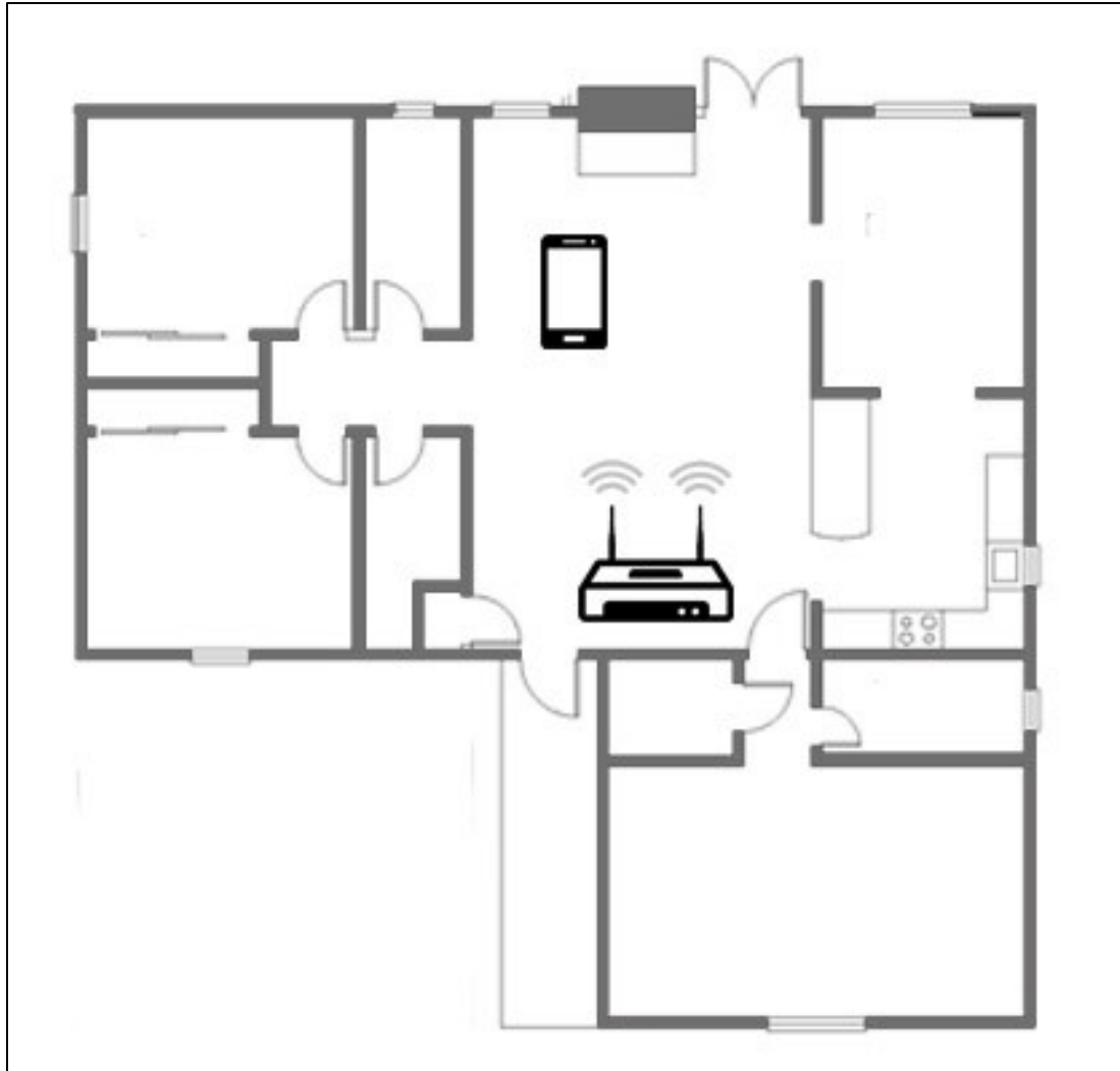
Figure 4.2: Location of a Smartphone and a single router in a 12 m 2 room of an apartment located on a partially constructed new building.
