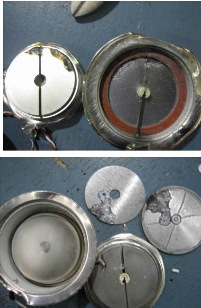
Figure 1.9: A damaged thyristor during a failure due to the temperature rise [12]
