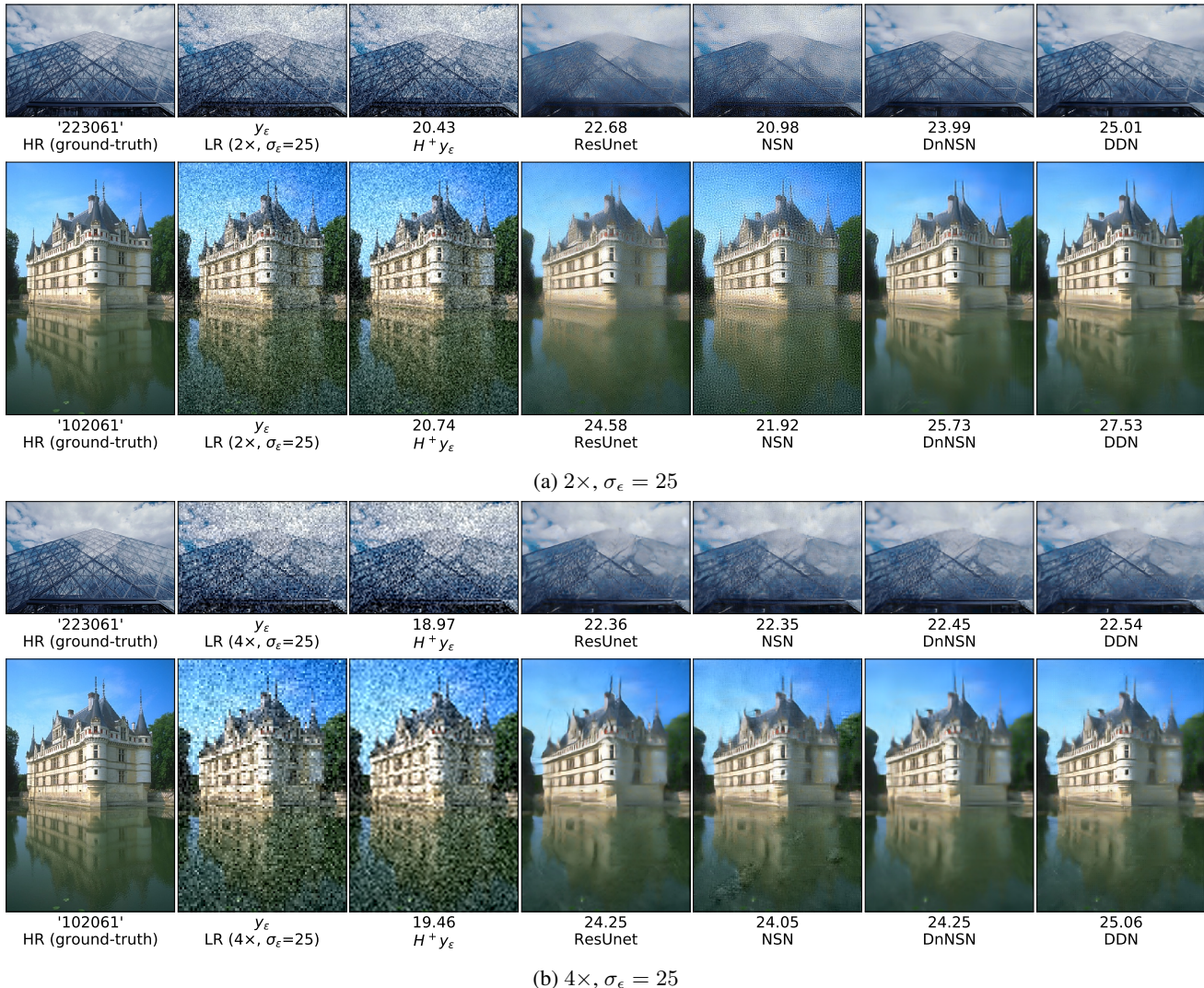
Figure 4: Visual demonstration and PSNRs of SR ( 2\times and 4\times ) results on the BSDS100 dataset with noise scale \sigma_\epsilon = 25 . From left to right: oracle image \mathbf{x} with its index number in the dataset, LR noisy measurement \mathbf{y}_\epsilon , bi-cubic upsample, results of ResUnet [15], NSN [35], DnNSN: DnCNN [44] + NSN, and results of the proposed method.
