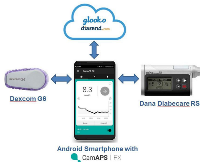
Figure 1 CamAPS FX app with Dexcom G6 sensor (Dexcom, San Diego, California, USA), Dana Diabecare RS insulin pump (Sooil Development, Seoul, Korea), and automatic upload capabilities to diabetes management system Diasend (Glooko/Diasend, Göteborg, Sweden) (reproduced with permission from CamDiab, Cambridge, UK).
