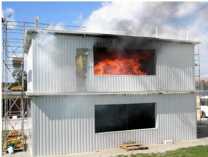
Figure 11. Experimental building during the Veseli Travelling Fire Test.
