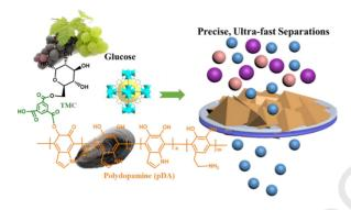
A facile technique to combine natural compounds and metal organic frameworks (MOFs) that produces a well-structured membrane with unparalleled separation performances was designed. Our synthesized membrane enables ultra-fast, low-pressure, precise separations for both solvent purification via organic solvent nanofiltration and desalination – key membrane-based processes for efficiently tackling worldwide water crisis.
