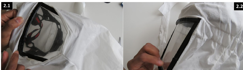
Fig. 6. (Left to right) Procedure to attach the curved face shield frame and helmet fitting to the SMS hood fabric.
