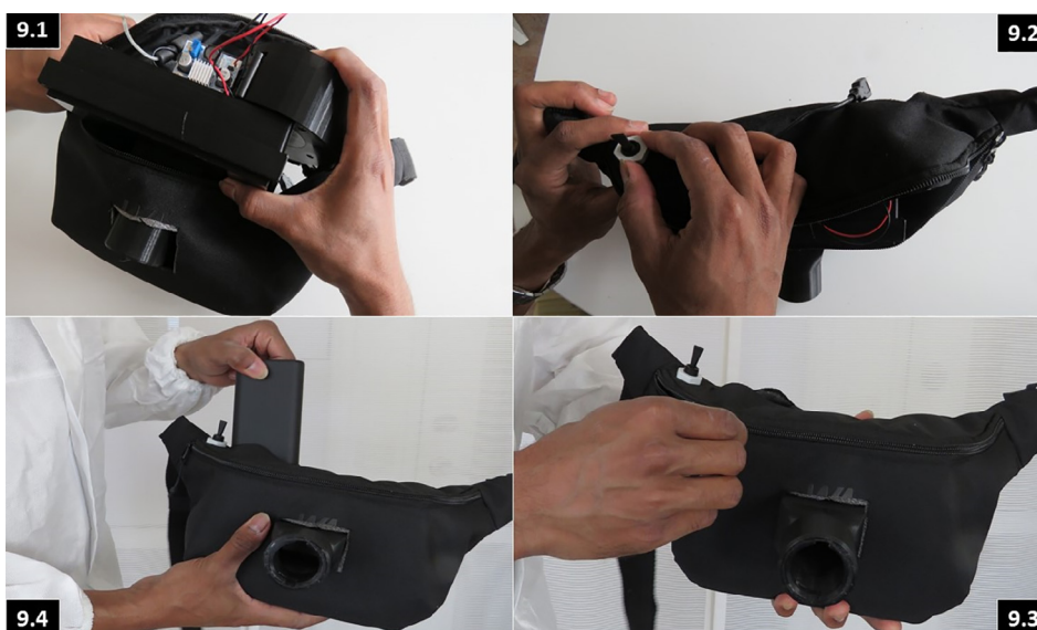
Fig. 14. (Clockwise) Procedure to place the FFU and power supply and conditioning unit inside the hip bag.
