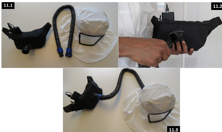
Fig. 16. (Clockwise) Procedure to connect the breathing tube between the hood and the FFU.
