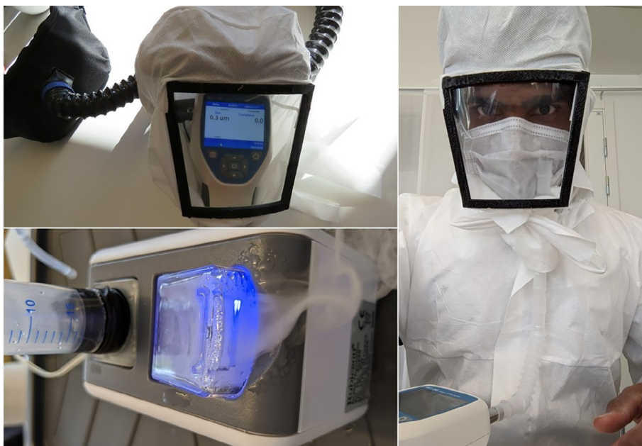
Fig. 20. Experiment setup to determine the particle count (left top) inside the hood of PROPER during operation without operator, and (right) with operator. (bottom) Humidifier used to produce the aerosol environment.
