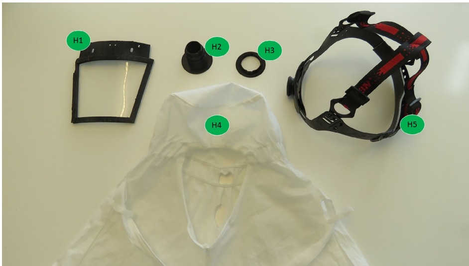
Fig. 4. Components for building the hood are denoted by their designator codes. H1 – Curved face shield frame, H2 – Hood adaptor, H3 – Hood adaptor flange, H4 – SMS hood fabric, and H5 – Helmet fitting.
