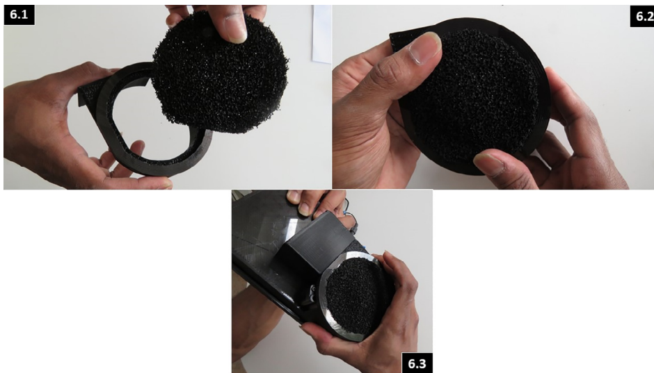
Fig. 11. (Clockwise) Procedure to secure the prefilter in front of the centrifugal fan.
