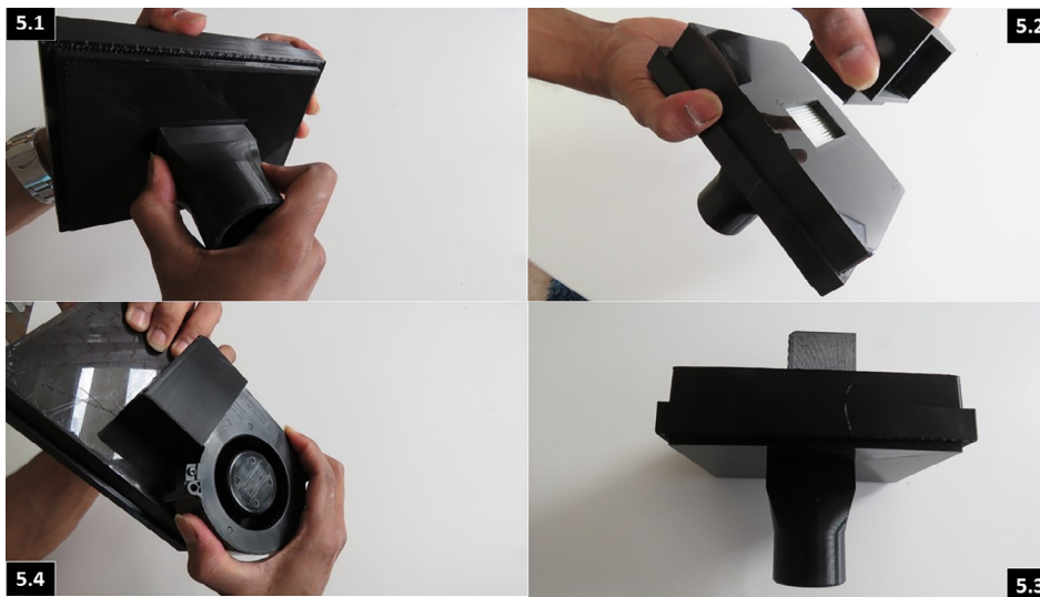
Fig. 10. (Clockwise) Procedure to secure the air pathway with adaptors and attaching the centrifugal fan.
