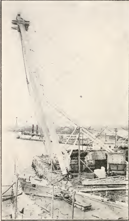
The immense shears used to load and unload boilers and heavy machinery on board war vessels, March 14, 1901.
