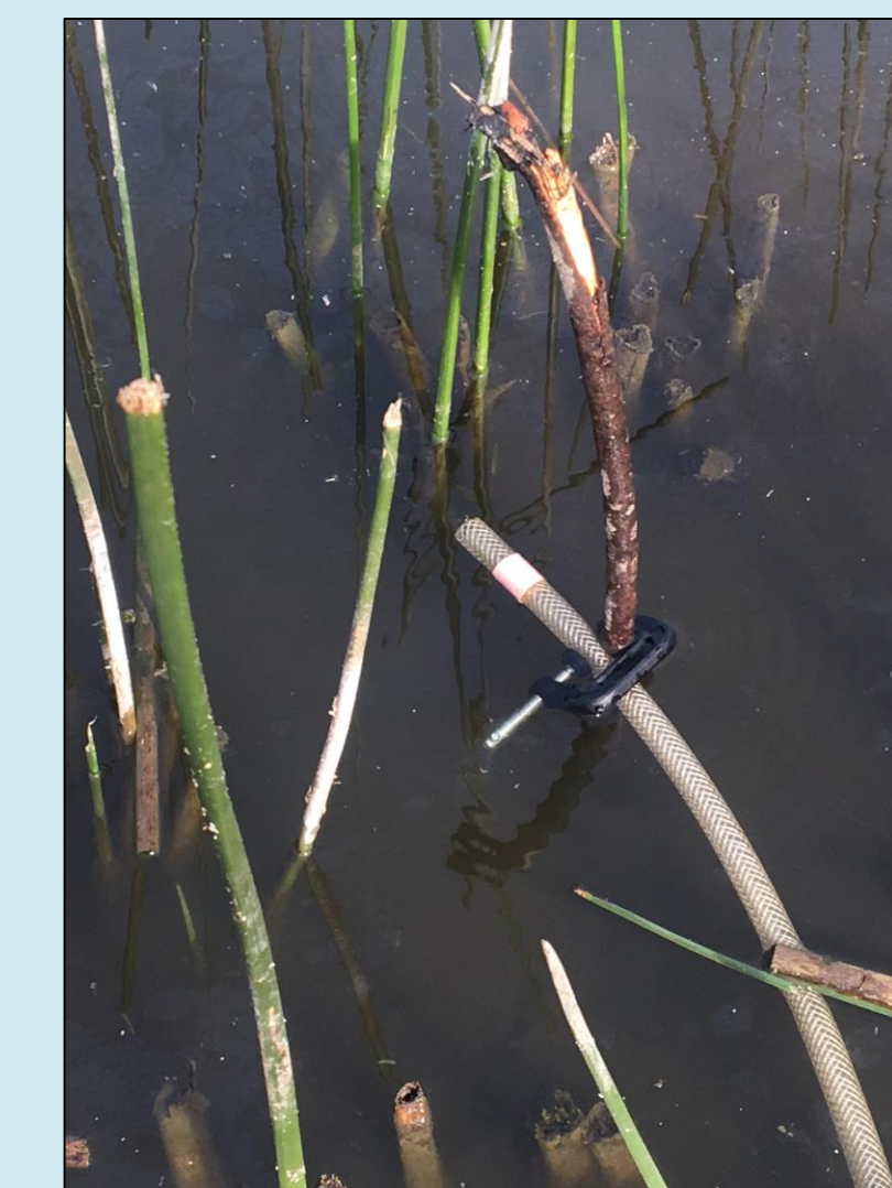
Figure 3. Tube held in place just below water surface where mosquito larvae live.
