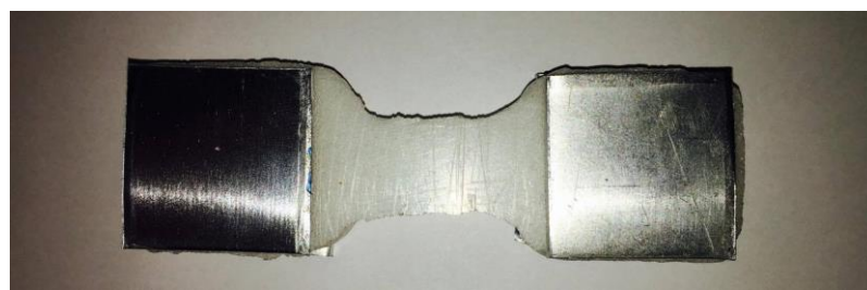
Fig. 21: Tensile sample with metallic parts
