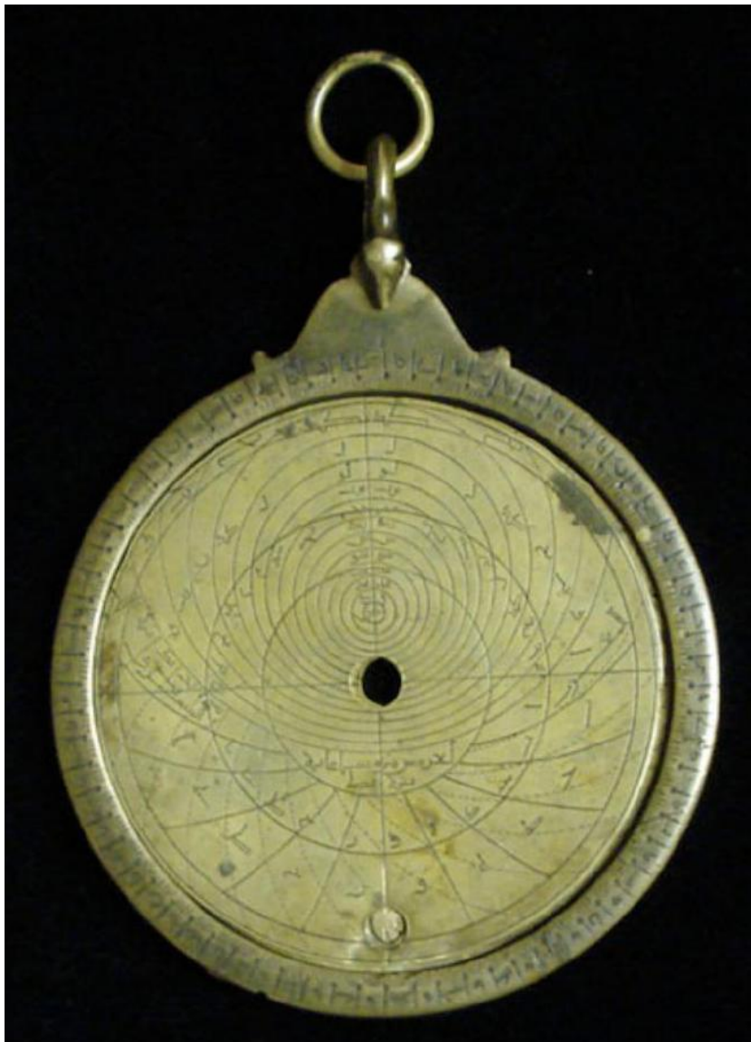
Fig. D1: The front of the astrolabe in the 'Abbāsīd tradition, showing the throne, the rim and the plate for latitude 45°.
