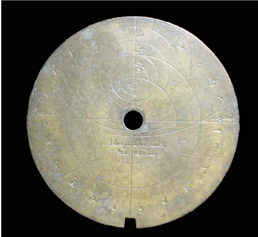
Fig. C1: The side of the plate for the third climate, corresponding to latitude 30°.
