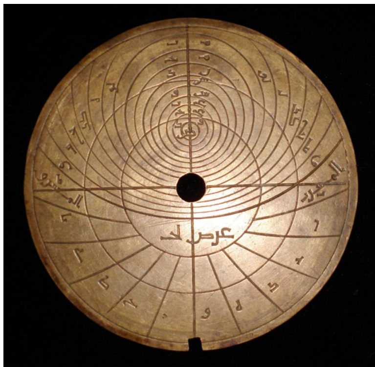
Fig. A4: The plate for 33°, which would serve Baghdad.
