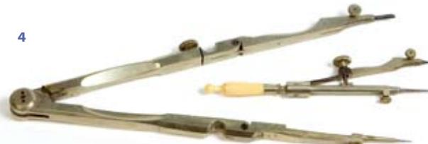
definitive form when, in around 1588, Swiss man Jost Bürgi inserted the regulating screw into the compass that allows the proportions of the arms to be modified at will. This screw slides along a groove that leads to a graduated scale to modulate the corresponding proportions.
