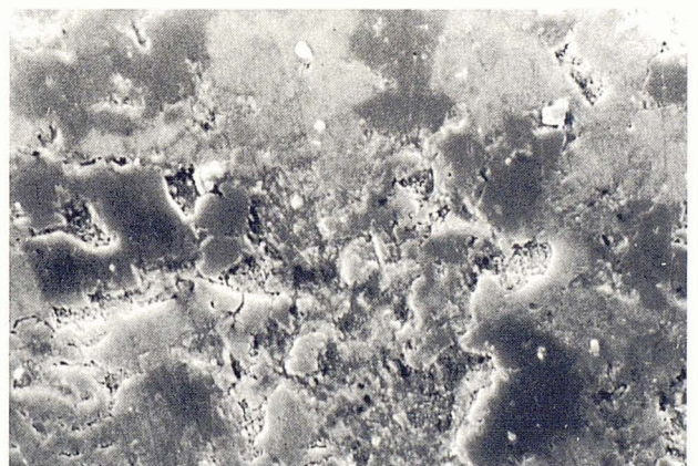
Figure 5: a) SEM showing surface area increase due to biological action (RK). Scale bars: 100μm and 20μm. b) Detail of polished surface of sample RP, showing irregularities which could be the incipience of a small quantity of carbonated particles. Scale bars: 100μm and 10μm.
