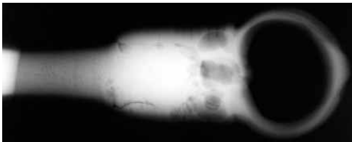
Figure 6.6: Micro-focus radiography of J-92 rein ring.
