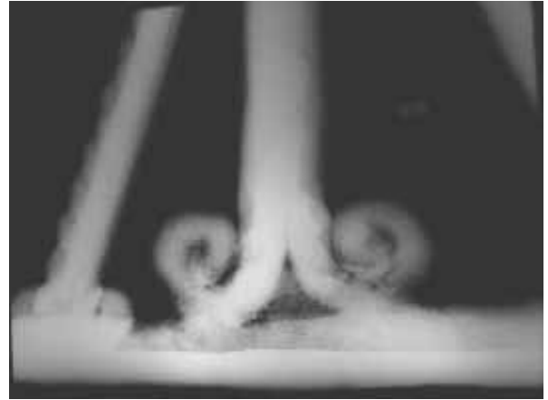
Figure 6.14: X-Ray radiography (Micro-focus) of J-60 base ring and leg.
