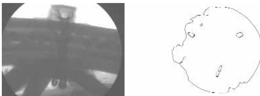
Figure 6.12: Micro-focus radiography of J-62 showing the ring, the rolled part of the «wire» and its open section just above the bowl, which became radio-transparent in the picture. On the right, line drawing showing top view of the bowl with the open, flattened wires (smaller scale than the photo).
