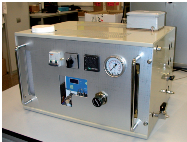
Fig. 5. Bio-ethanol reformer equipped with catalytic monoliths and a separation membrane selective to hydrogen. The permeate is hydrogen of high purity that can be feed directly into a low-temperature fuel cell for mobile applications.
