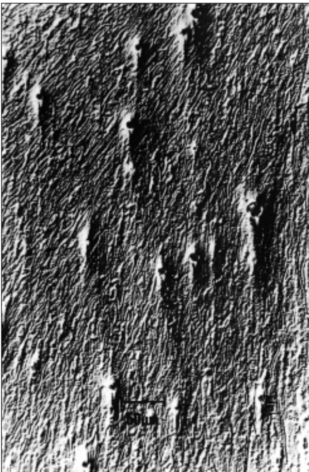
Figure 6. Cellular microstructure obtained by gravity casting commercial magnesium into a cylindrical copper mould. Second phase particles were detected as Fe-rich particles [43].
