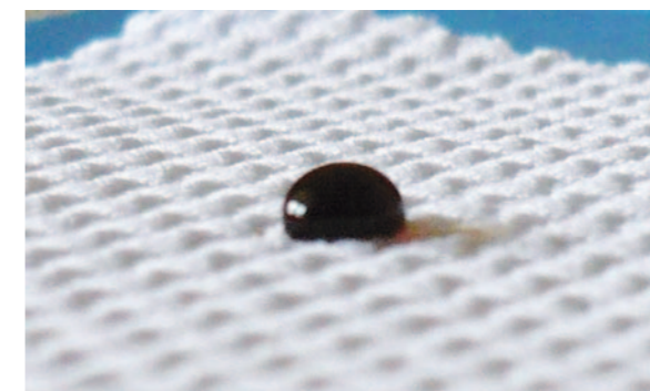
▲ These fabrics have a fluorocarbon-based surface finish that provides the finished side with superior hydrophobicity or water repellency
