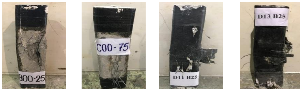
Fig. 2 – Failure of controlled and BFRP strengthened specimens.
