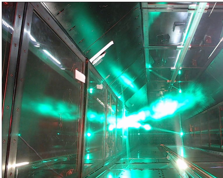
Figure 10.12: Image from a conventional camera taken during a typical experiment looking upstream. The overexposed parts of the green laser beam are regions of high particle density. Note that the laser beam was wider during this experiment than described here. The measurement volume is above the white light visible in the front of the picture.
