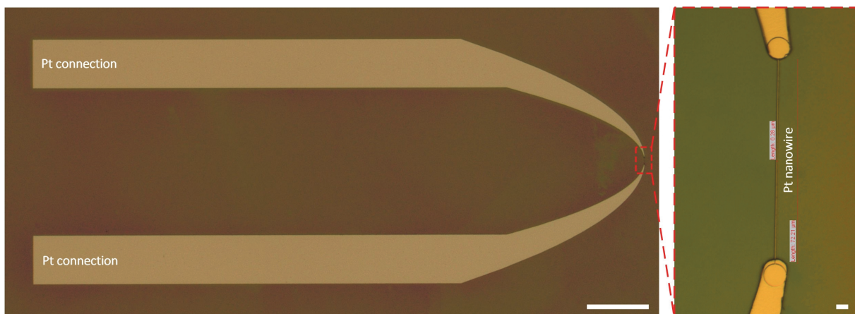
Figure 3 Optical microscopy image (scale bar: 500 \mu\text{m} ) of Pt connections, with a close-up image at the Pt nanowire location (scale bar: 5 \mu\text{m} ).
