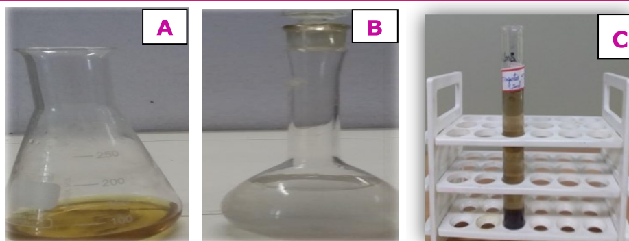
Fig. 2. Green Synthesis of silver nanoparticles from Tagetes leaves extract. Note: A = Tagetes leaves extract before adding AgNO_3 , B = Silver Nitrate solution., C = Tagetes leaves extract after 20 min of incubation.
