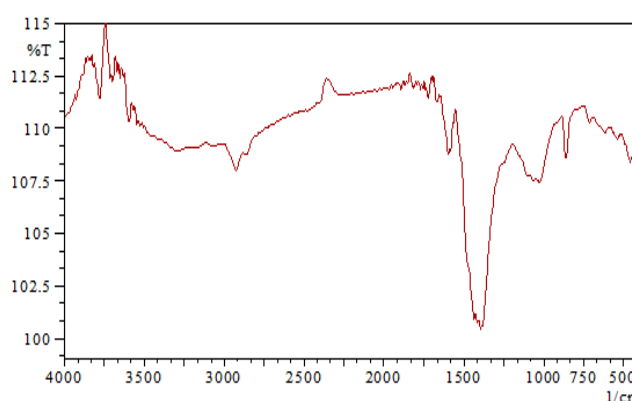
Fig. 4. FT-TR spectra for Tagetes erecta leaves extract reduced silver nanoparticles.
