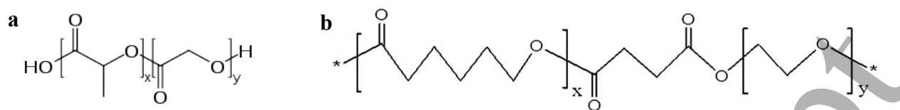
Figure 1. Chemical structures of (a) poly(lactic-co-glycolic acid) (PLGA) ( x is the number of lactic acid units and y is number of glycolic acid units) and (b) PCL- b -PEG ( x is the number of caprolactone units and y is number of ethylene glycol units).
