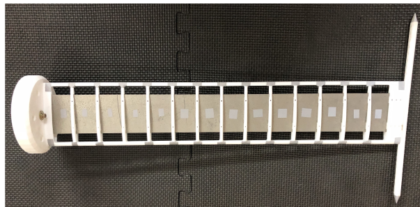
Fig. 10 Pazy wing experimental model.
