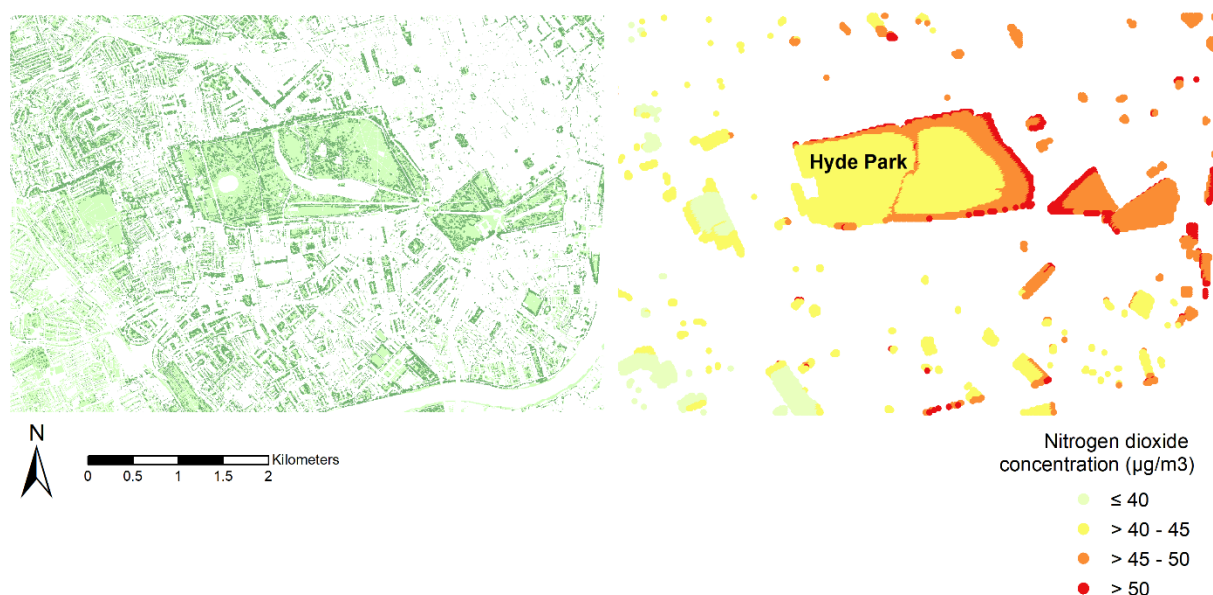
Figure 4. Vegetation cover (GeoInformation Group data) in Hyde Park, London, and the surrounding area (left panel) shown with modelled nitrogen dioxide concentrations (London Atmospheric Emissions Inventory, 2016, 20 m x 20 m grid square centroids) within vegetation cover (e.g., Hyde Park) boundaries (Ordnance Survey Open Greenspace data; right panel).
