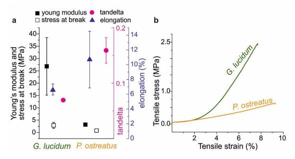
**Figure 1.4**. Mechanical features of mycelia. (a) Young modulus, stress at break and elongation results after the tensile test; tanδ values after DMA analysis. (b) Tensile test curves of the two mycelia under study.
