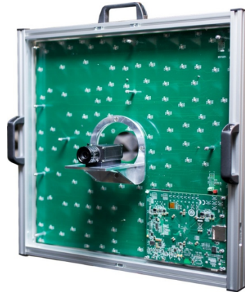
Figure 5.1 Acoustic images are obtained from a geometrically structured array in which microphones are embedded in a single compact device called Dual Cam . Dual Cam is a prototype made of 128 microphones, 50 cm x 50 cm, working in real time over a wideband (500 Hz–6400 Hz). Microphone layout and processing parameters are optimized according to a patented method. Frame rate: 12 frames per second. Maximum field of view: 90° elevation, 360° azimuth (tunable according to the video camera field of view). State of art beamforming algorithm: robust, superdirective filter-and-sum beamforming.
