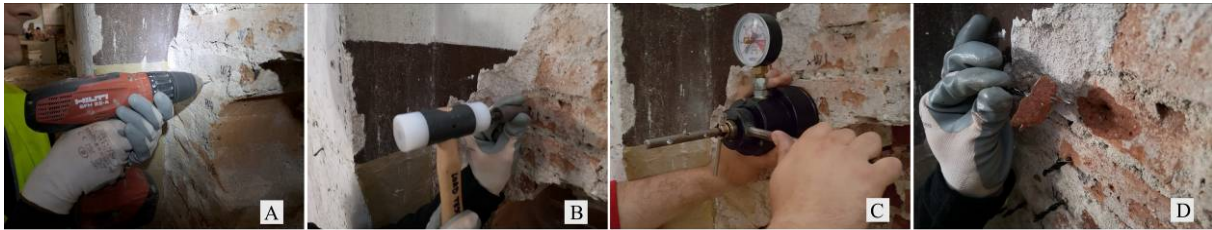
Figure 2: Helix Pull-out Test operation: (A) drilling the pilot hole, (B) hammering the tool until the helical tie is introduced in the pilot hole, (C) loading by turning the grip lever until failure, (D) failure in the brick.
