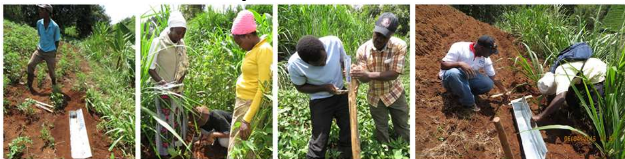
Figure 2: Photographic representation of the soil trough setup in the various plots: (1st LEFT) A soil trough installed in one of the plots with beans and Napier grass; (2nd LEFT); A CGIAR-WLE Scientist training farmers on how to read and record data from a calibrated runoff detector soil trough; (2nd RIGHT): CGIAR-WLE Scientist installing a rain gauge in one of the farms (RIGHT); CGIAR-WLE Senior Scientist supervising the installation of the soil troughs in designated experimental plots (Photo Credits, Fred Kizito).
