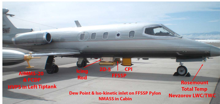
Figure 15. The approximate locations of the 11 instruments carried by the SPEC Learjet during SEAC 4 RS. All the instruments make in situ measurements. Photo courtesy of Paul Lawson.
