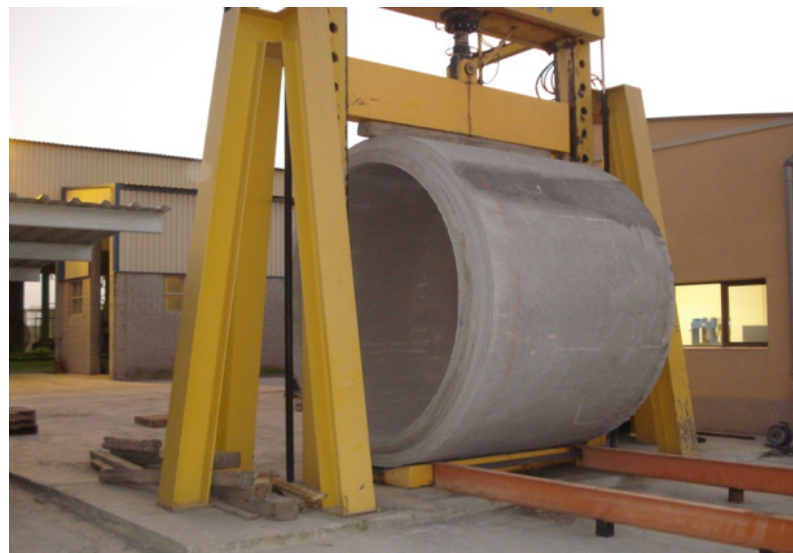
Figure 1. Three-edge bearing test on a 2500 mm double-cage steel reinforced concrete pipe.
