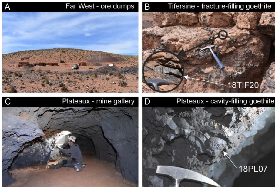
Figure 6.2.5. Field pictures of Imini district. (A) Far West site ore dumps. (B) Botryoidal goethite filling fractures and forming thin veins, at Tifersine site (sample 18TIF20). (C) Mine gallery at the Plateaux site. (D) Large botryoidal goethite filling cavities at the Plateaux site (sample 18PL07).
