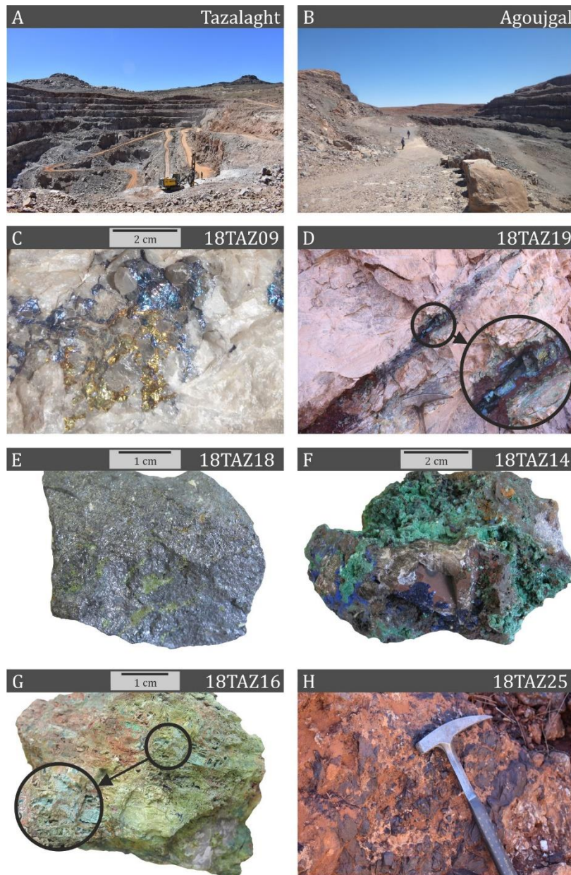
Figure 5.3.4. Field pictures of Tazalaght and Agoujgal, and representative Tazalaght's samples pictures. (A) Tazalaght open-pit quarry; (B) Agoujgal open-pit quarry; (C) Primary sulfides (chalcopyrite, bornite) filling cavities in quartzite; (D) Secondary sulfides (bornite, chalcocite), malachite, and goethite, in stratabound vein in Tamjout dolomite; (E) Slightly weathered tennantite; (F) Malachite and azurite filling cavities in quartzite; (G) Cu-arsenates (mostly olivenite) replacing tennantite with a boxwork texture, in cavities in quartzite; (H) Gossan hosting massive goethite, in quartzite.
