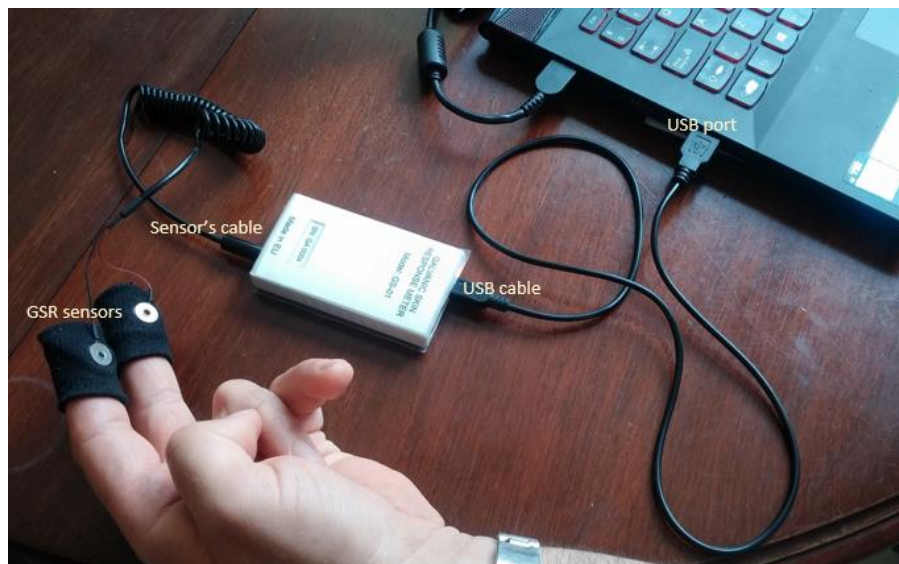
Figure 9. Usage of a GSR measuring device
