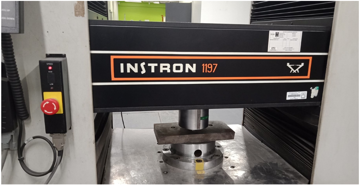
Figure 11 Instron Compression Testing Machine
