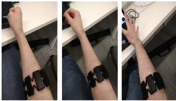
Figure 2. Defined gestures for electromyographic data acquisition. The fist is either clenched [left], splayed open [right], or returned to a neutral position [centre].
