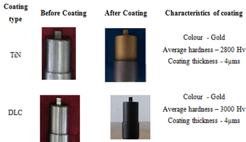
Fig. 3 Tools with coating characteristics
