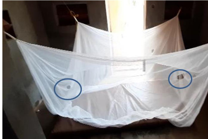
Figure 4.7: Net holed according WHO recommendations. Six holes (4 cm × 4 cm) per net, two on each of the long sides and one on each of the short sides.
