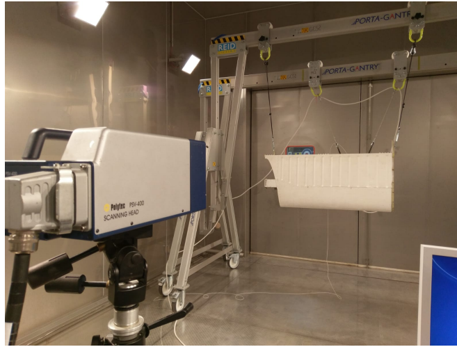
(a) test-rig and scanning laser vibrometer
