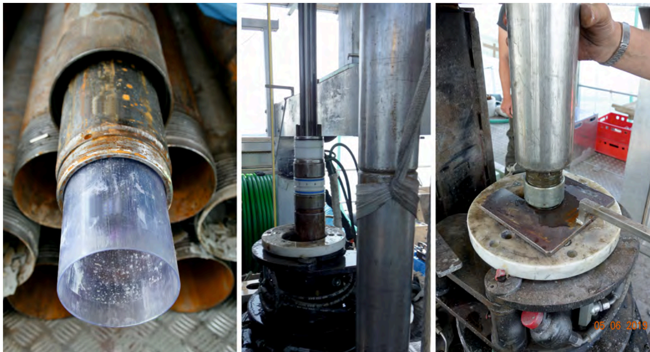
Figure 4: Casing, core barrel and inner liner before set up (left), coring assembly lowered into lake with connection of core barrel with DHT-hammer atop in the rotary unit (middle) and heavyweight rods above the hammer unit hold in place in rotary unit through a make-up plate (right).
