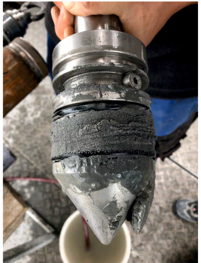
Figure 5: Opening of the coring barrel with view on 1.85 m long, core-filled plastic liner (grey) and core catcher (white) (upper); piston in the core-filled upper end of the liner (lower left); piston after core retrieval with sandy sediment from Lake Constance (lower right).
