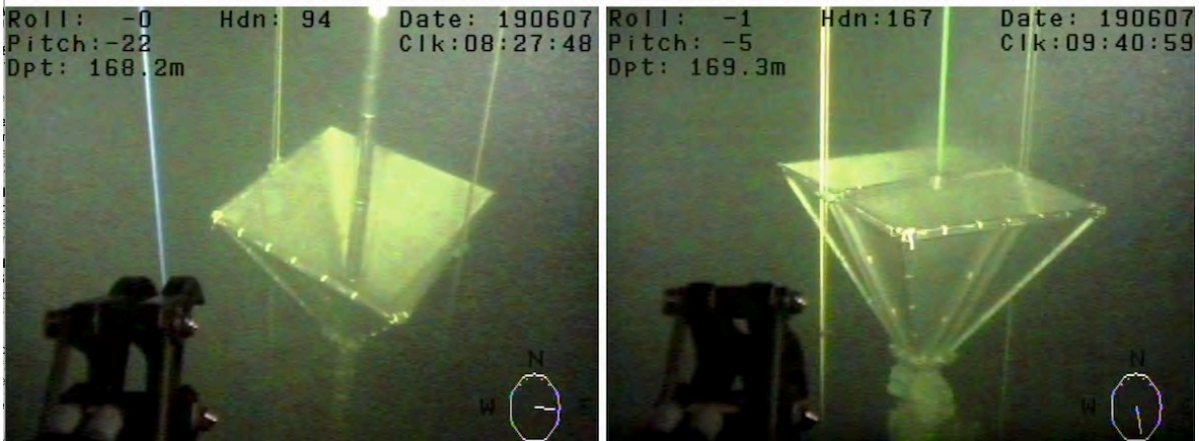
440 Figure 2: Hipercorig on Lake Constance during coring operations in 2019, upper panel; video stills from R/V Kormoran ROV showing entry of coring assembly in the upper re-entry cone, lower left panel, and re-entry cone with hydraulic hose (green) after coring assembly was lowered into the hole, lower right panel.
