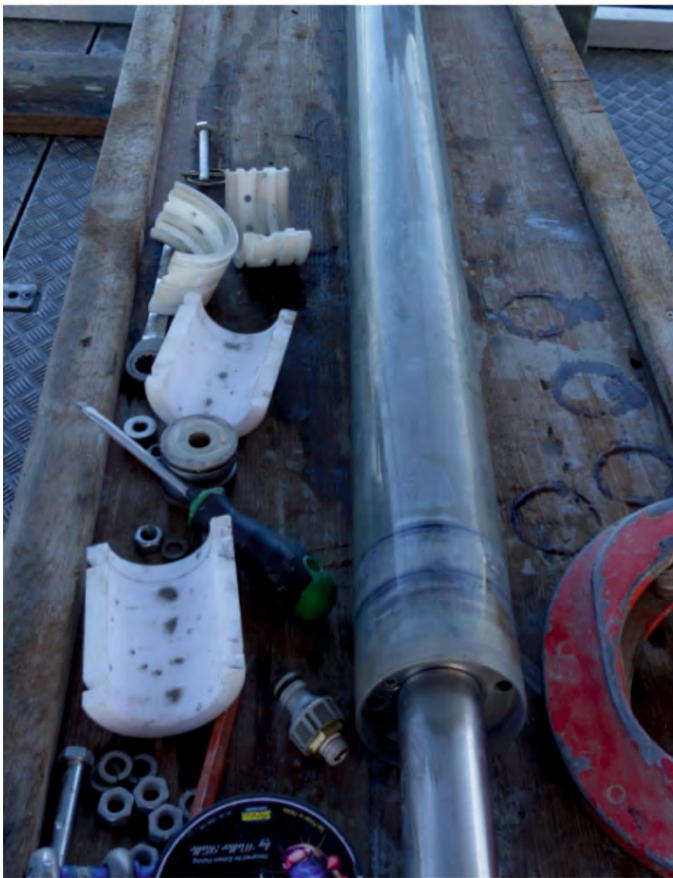
Figure 5: Opening of the coring barrel with view on 1.85 m long, core-filled plastic liner (grey) and core catcher (white) (upper); piston in the core-filled upper end of the liner (lower left); piston after core retrieval with sandy sediment from Lake Constance (lower right).
