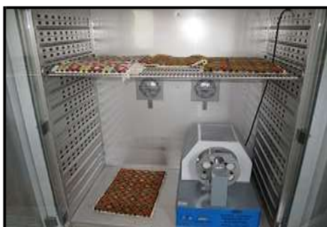
Figure 12. Putting samples under bad conditions of temperature and humidity
