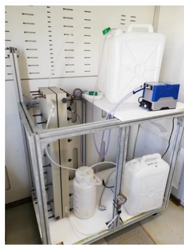
Figure 2-2 Schematic representation of the continuous experimental systems. (a) balances, (b) peristaltic pumps, (c) Diffusion Dialysis units, (r) retentate buffer, (d) diffusate buffer, (f) feed tank, (w) deionized water tank, (P) pressure meter. The arrows have the same meaning of Figure 2-1 (on the left); picture of the real DD large laboratory experimental set-up (on the right).
