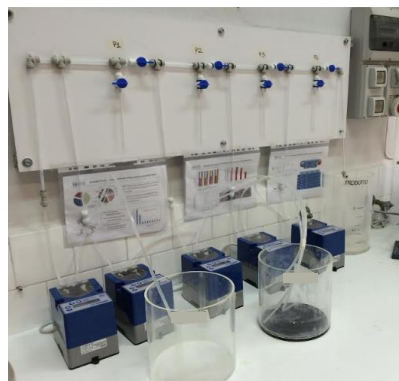
Figure 3-4 Schematic representation of the PFR reactor (on the left) and laboratory PFR experimental set-up picture (on the right).
