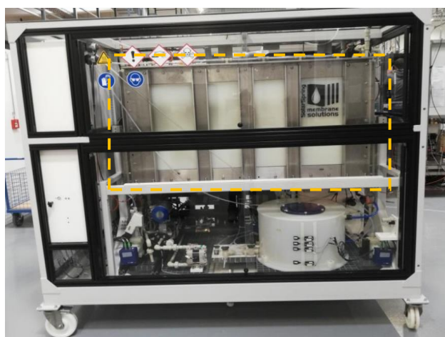
Figure 5-7 Back view of the demonstrator plant. MD unit is marked with a yellow rectangle.
