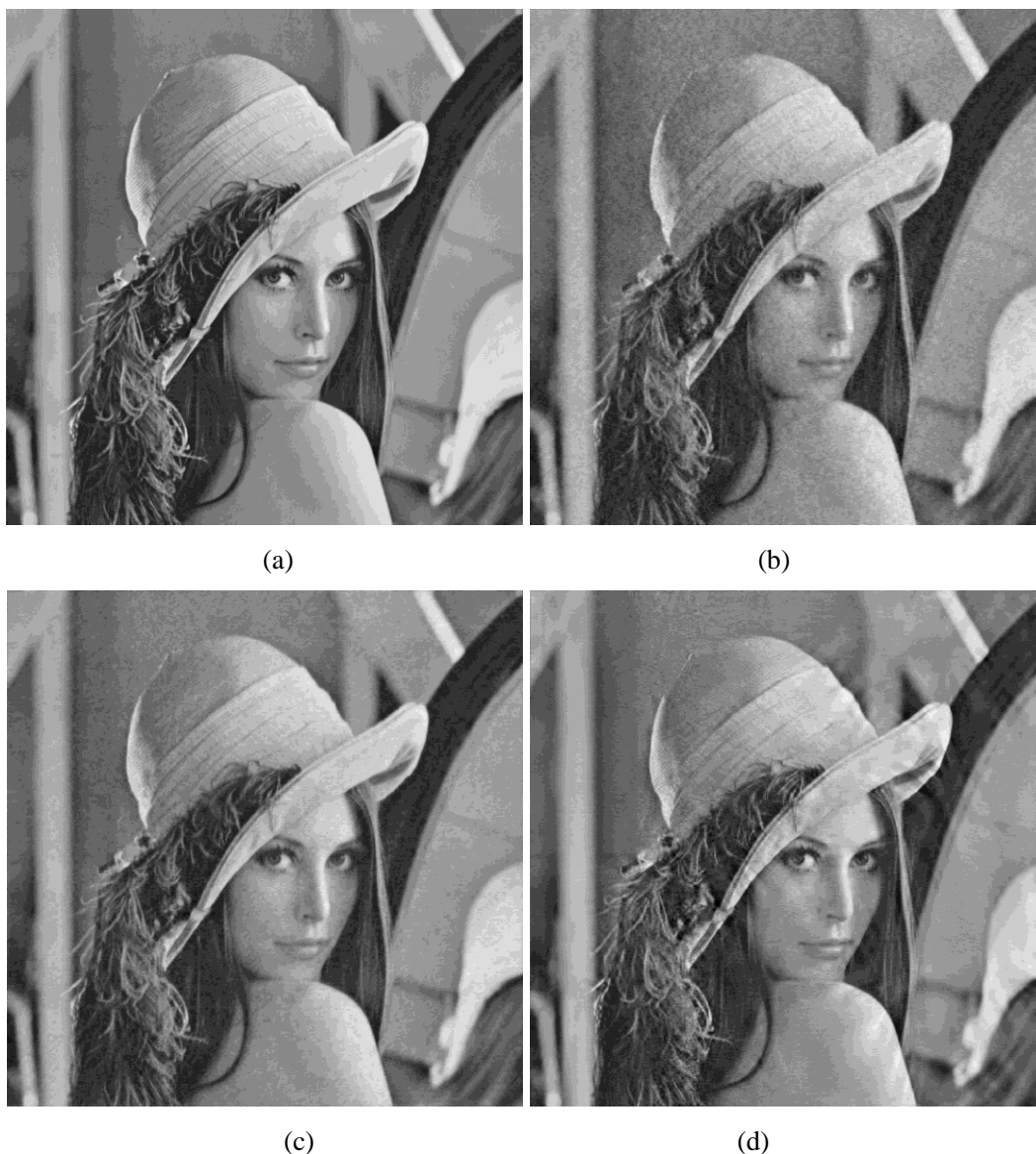
Figure 4- 5. (a) Standard photo image-Lena ( 512 \times 512 pixels) and images reconstructed by using 50% data and CS-SPGL1 approach with (b) DCT sparse basis (c) FFT sparse basis and (d) Haar-DWT sparse basis
