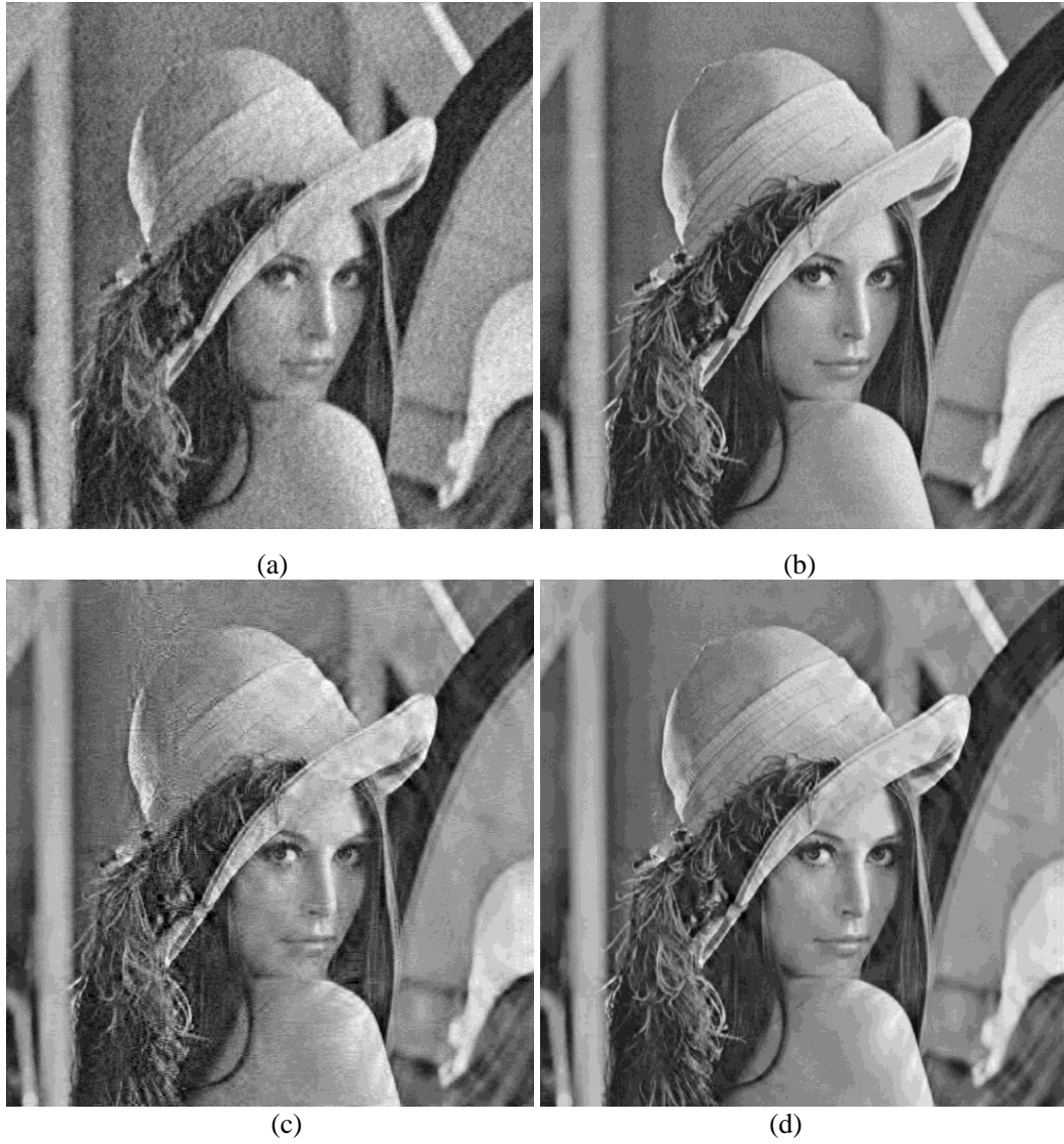
Figure 4- 6. Lena images reconstructed by using the CS-OMP approach with FFT sparse basis. (a) 40% data (b) 70% data and Haar-DWT sparse basis (c) 40% data (d) 70% data
