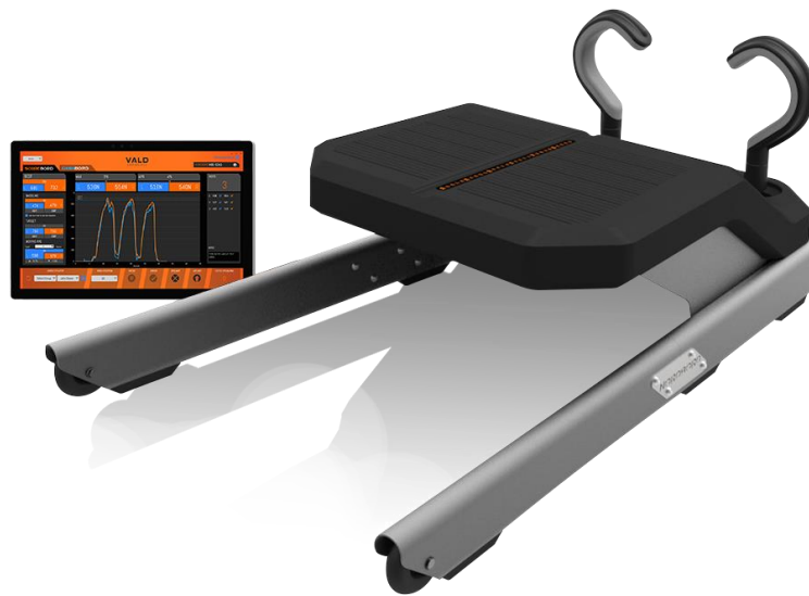
Figure 1. NordBord Hamstring Testing system.
