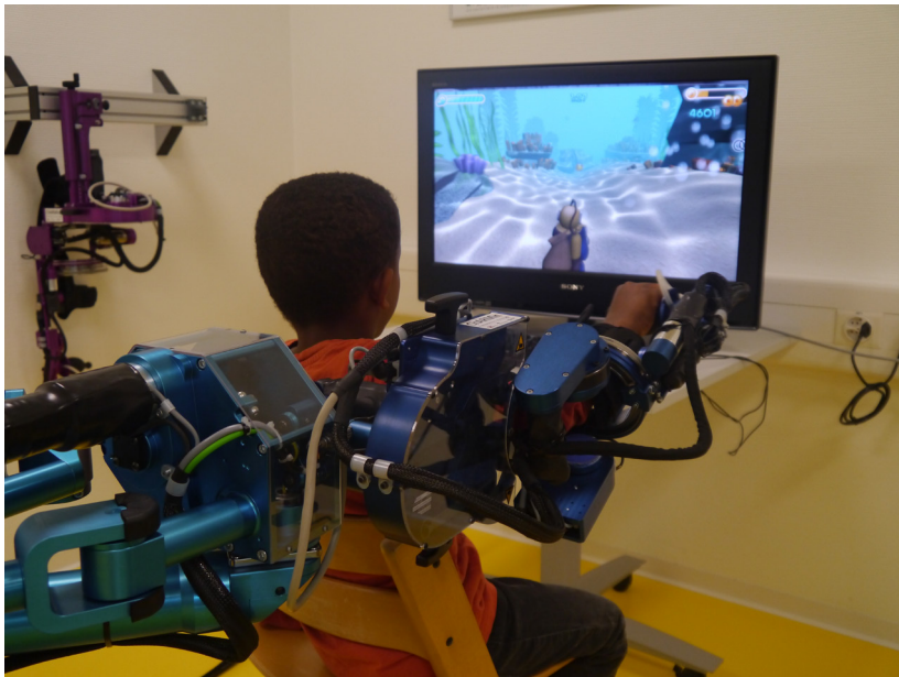
Fig. 5.2. The ChARMin robot. The ChARMin exoskeleton: A young boy practicing with ChARMin's small distal module.
