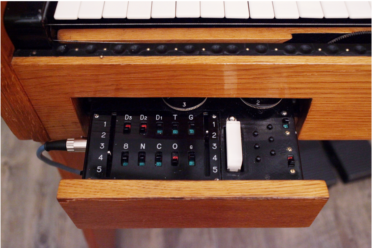
Figure 5. The drawer or tiroir . The left half has switches for timbres and loudspeakers. Sliders (with numbers from 1 to 5) are volume controls for the octaviant (left) and the petit gambé (right). Dial wheels are balance adjustments for the loudspeakers (left) and the souffle (right). The rightmost switches are the souffle (top) and the ribbon/keyboard selector (bottom). The left side of the drawer has a switch for the loudspeaker D4, and a cable connector for the pedals.
