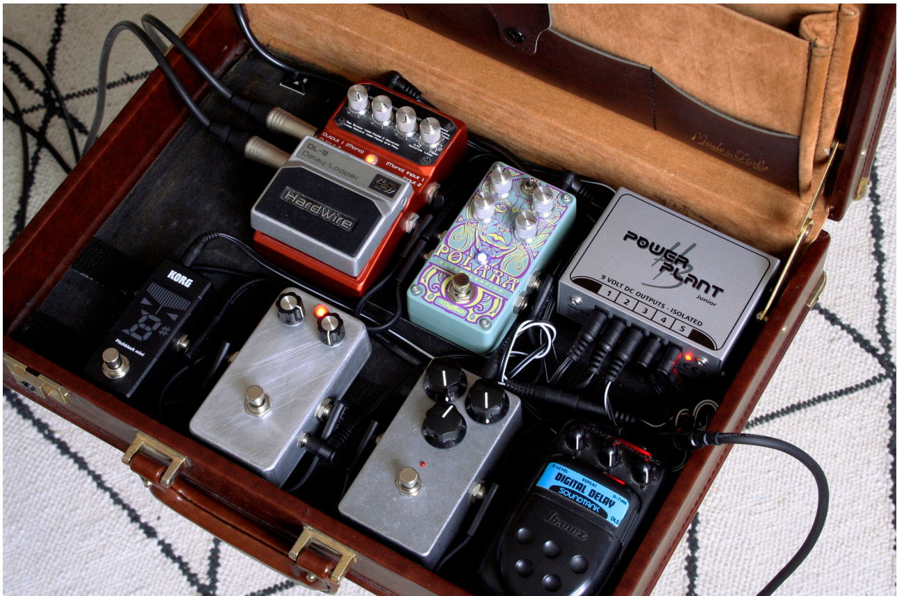
Figure 11. The briefcase pedalboard. Top row, from left: Digitech Hardwire DL-8 delay and looper, Digitech Polara reverb, and Harley Benton PowerPlant Junior power supply; bottom row, from left: Korg Pitchblack Mini tuner, DIY fuzz, UralTone kit tremolo, and Ibanez Soundtank DL5 delay.
