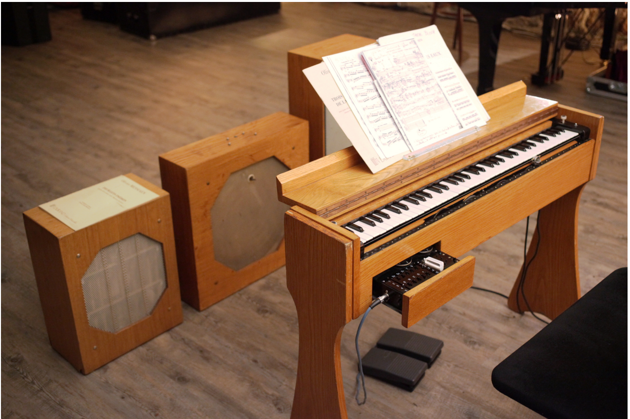
Figure 1. Thomas Bloch's Ondes Martenot (seventh model, built in 1985) with three of its loudspeakers or diffuseurs .
