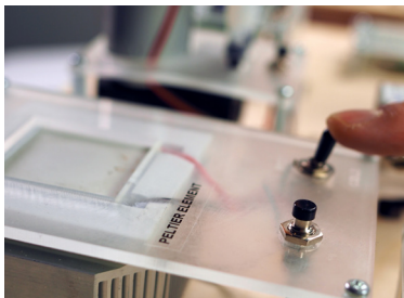
H/ Thermoelectric Cooler Module. Switch: set cold or hot. Button: activate.
