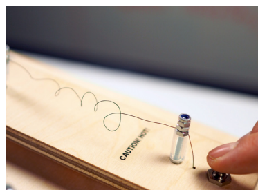
M/ Shape Memory Alloy. Button: Move alloy to original shape.
