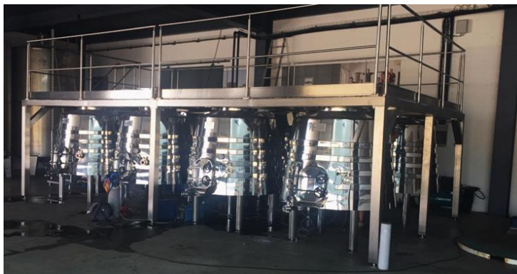
Figure 2.4 – Pilot unit placed in Herdade da Malhadinha Nova cellar, composed by eight fermentation vats (four in the front and four in the back).
