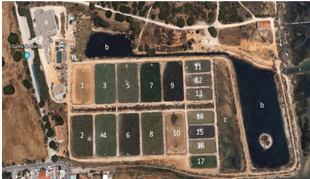
Fig. 1 - Aerial view of the Aquaculture Research Centre (EPPPO, IPMA) facilities localization and spatial layout: a – Hatchery; b – Reservoir; c – Settling pond; 1-17 experimental earthen ponds
